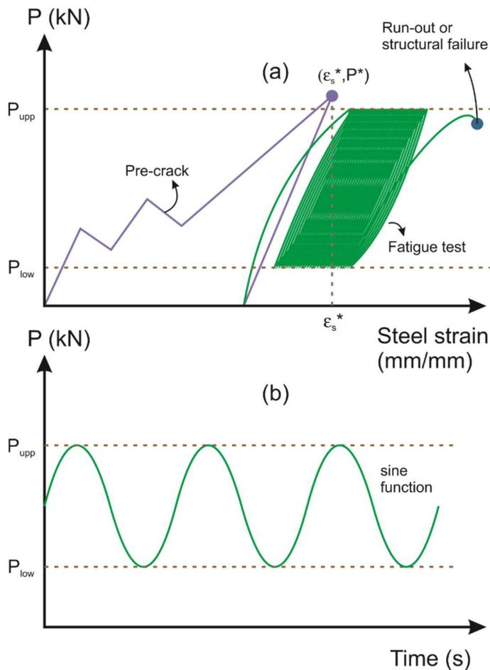
Figure 3: Fatigue test program: (a) test stages from the pre-crack until the fatigue loading and (b) loading oscillation at 6 Hz of frequency.
