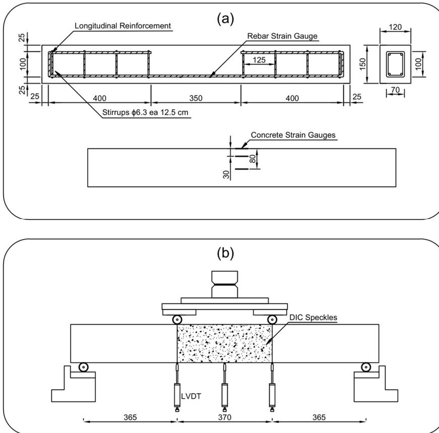
Figure 2: Setup illustration: (a) reinforcement configuration and gauge positions and (b) setup with LVDTs disposal. Dimensions in mm
