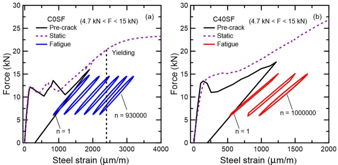
Figure 4: Fatigue longitudinal rebar strain evolution, quasi-static and pre-crack results for (a) C0SF and (b) C40SF under the same fatigue loading range.
